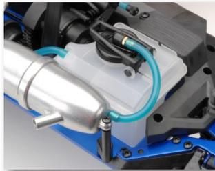
**Aluminum Manifold and Muffler** – Monster trucks need to be tough, and the exhaust system is no exception. The MFR includes a rugged aluminum manifold and muffler, which can handle more punishment than a plastic exhaust system, and it helps to increase the performance of the already-powerful GXR18 engine.
