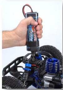
**Touch Start System** – Electric starting was never so easy as it is with the on-board “Touch Start” system included with the MFR. Simply attach the included connector unit to any 6-cell Ni-MH or 2-cell LiPo battery pack and press the connector into the touch starter unit. There’s no locking plug or latches, so you don’t have to worry about the truck driving away with your battery pack attached, once the engine is started, simply lift the battery/connector unit and drive away.
