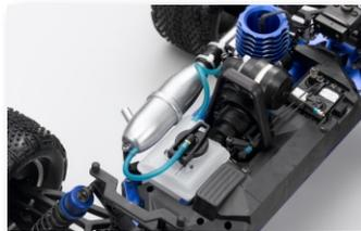
**Triple-Deck Chassis** – The front and rear bulkheads attach to the chassis via the top and bottom deck, and the distance between the two attaching points provides superior strength and rigidity so you can take the biggest jumps with confidence. The middle deck is home to the powerful GXR18 engine, electronics and the dynamic QRC transmission.
