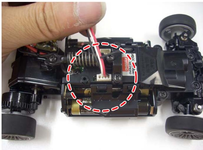
4. While pushing the pairing switch down, turn the power ON.
