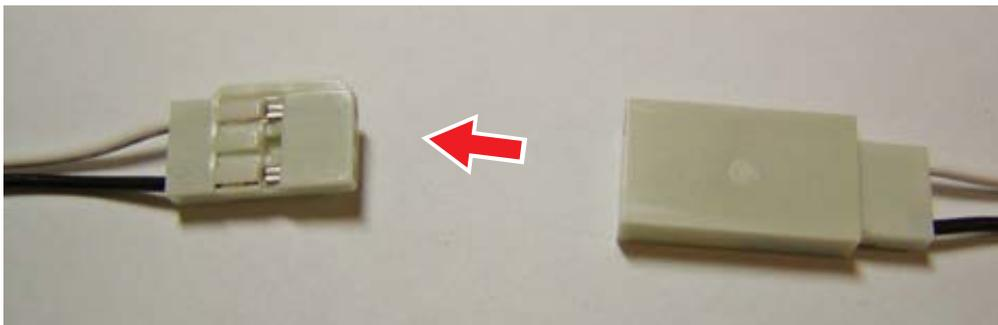
3. Connect the I.C.S. Cable to the I.C.S. Connector on the (Mini-Z or dNaNo) model.
