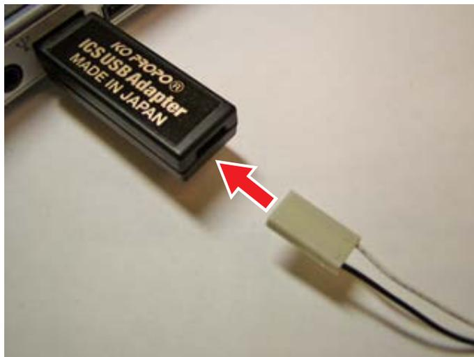
2. Connect the I.C.S. Cable to the Extension Cable.
